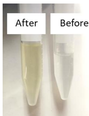
Figure 3.8 Photographs of product after plasma treatment and feed solution
