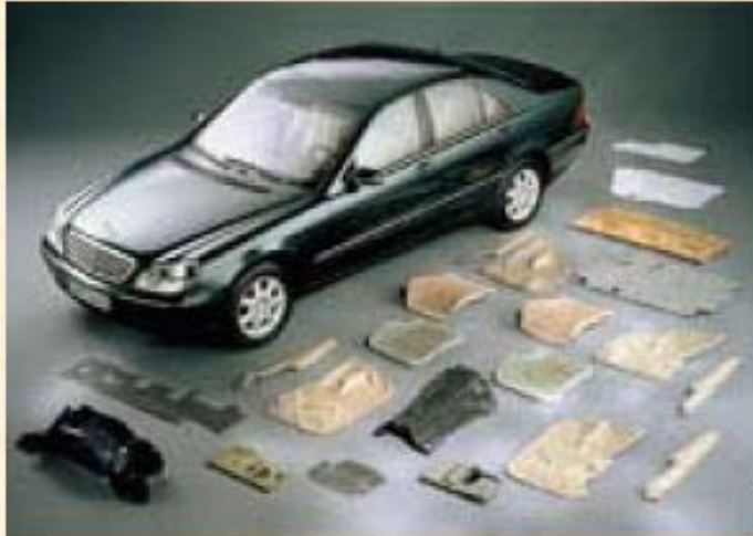
parts of the Mercedes-Benz S-Class that are made from natural fiber reinforced composite material.
